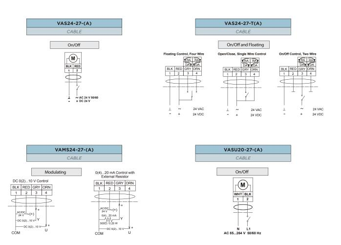
Important - Do not install multiple VAS-27 Series actuators connected to the same mechanical load. Master-Slave application of DS-27 Series Actuators requires that each actuator be connected to independent loads.
